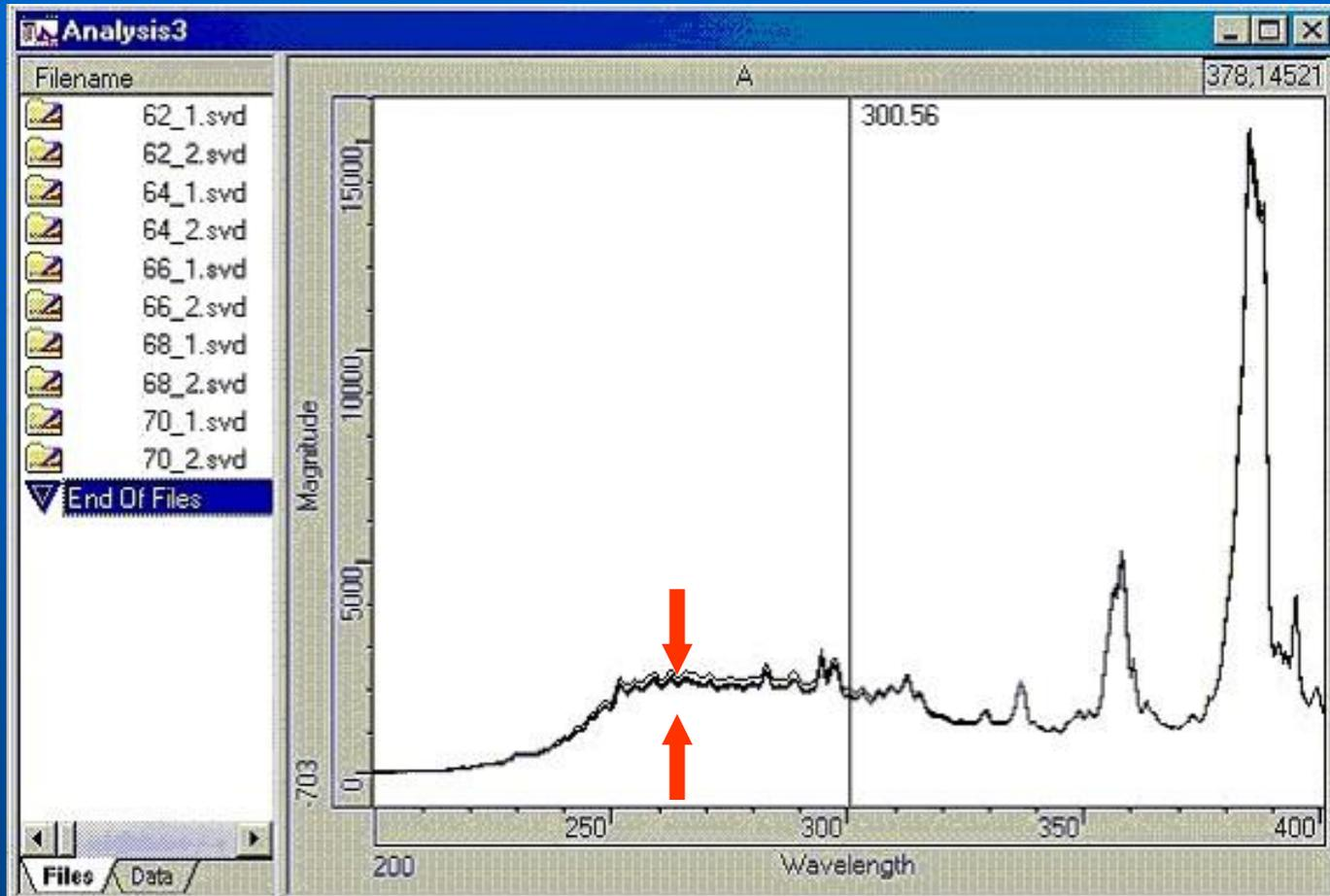
Calibration with UV-visible spectra is degraded by window clouding, which causes small changes that are greatest in UV and least in red.
