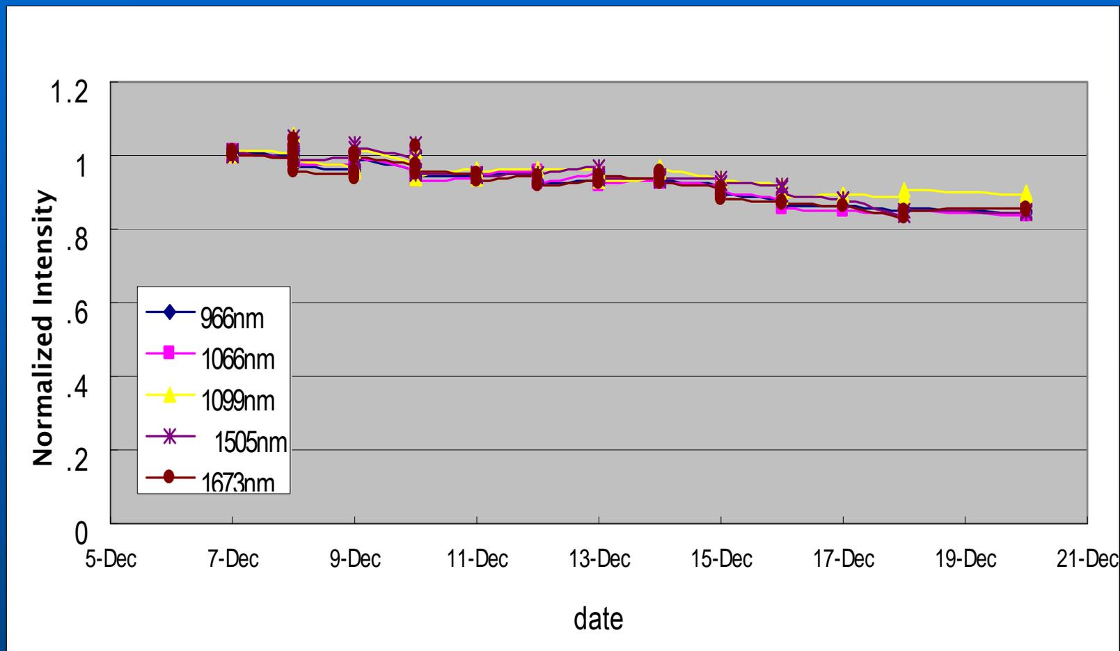
Verified that window transmission is greater in Near-IR and spectral intensity decreases in time less than in UV-Visible region.
