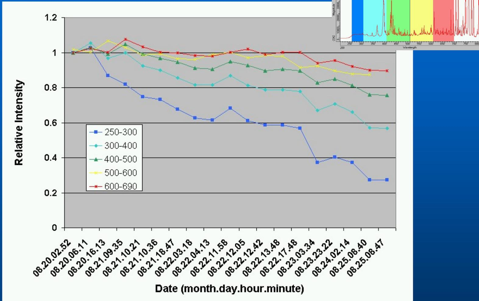
The intensity of the UV-visible spectra decreases in time more in the UV spectral region and less in the red region.
