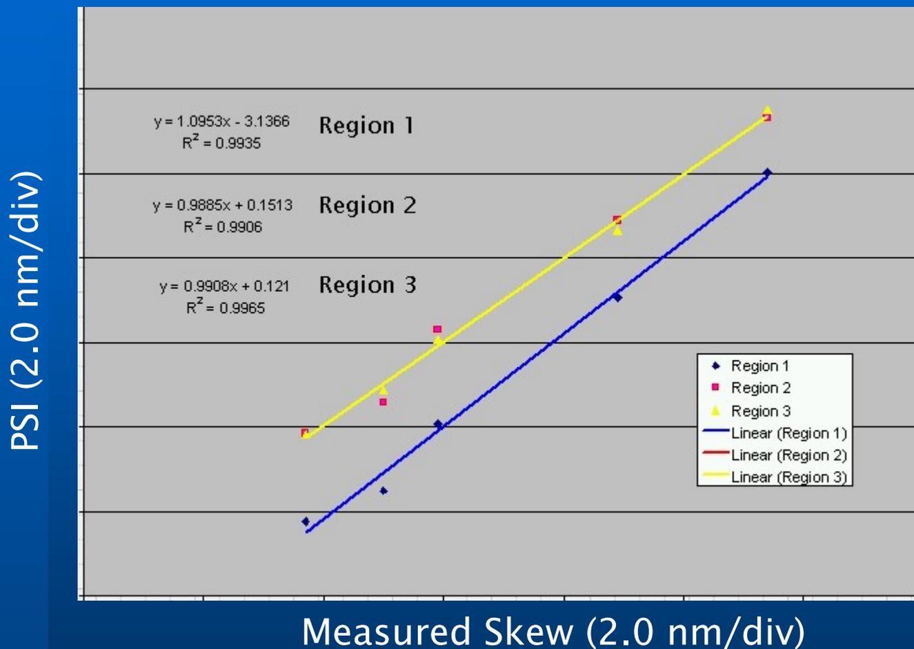
PLS Calibration with NIR spectra and the measured skew of the etched wafers
